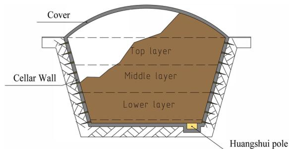
**Fig. 1** A diagram of a CSFB fermenting cellar
